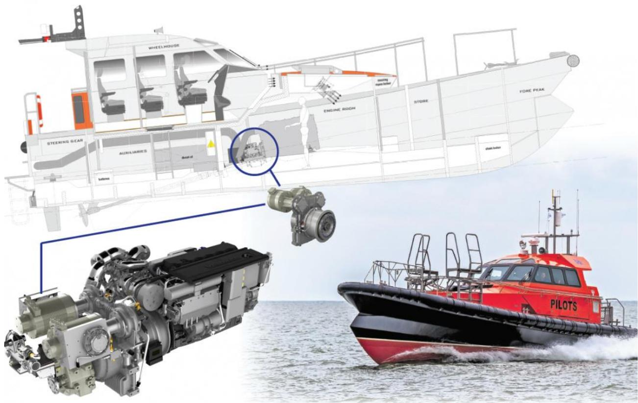
The new hybrid pilot boat by Goodchild Marine Services Limited mounts a plug-in parallel hybrid propulsion system by Transfluid.
