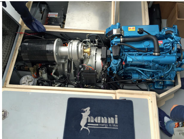
The 20 kW HTM700 model coupled with the Nanni Diesel. The electric motor is black and on the left.
