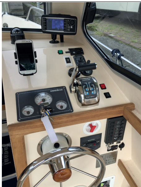
The command station of the launch with the Flexball control lever.
