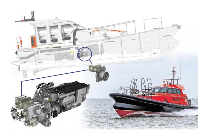
The new hybrid pilot boat by Goodchild Marine Services Limited mounts a plug-in parallel hybrid propulsion system by Transfluid.
