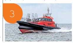
1. Each of the new boats will be 24m long with a displacement of 90 tons
