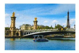
Two electric passenger boats are operating on the Seine in Paris. The boats can carry up to 12 people plus the skipper and have a range of 24 hours. They are 8.30m long and 3m wide. Propulsion is provided by the Bellmarine/Transfluid electric system with two 15kW
